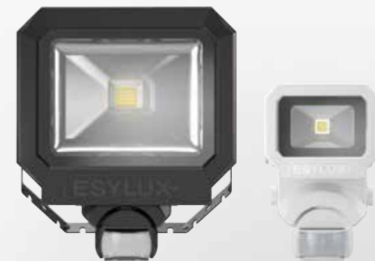
▲ The built-in motion detector in the AFL SUN floodlight reduces operating costs and extends the service life of the LEDs.
